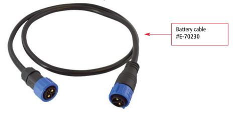
IDENTIFICATION Both connectors are blue Tool side : 8 pins Battery side : 2 pins
