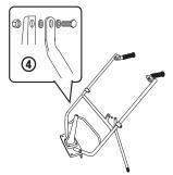
5- Assembly of the engine Remove the engine from the protective foam.Place the engine on the housing shaft, make sure that the driveshaft is inserted in the clutch adaptor, and tighten. (Do not overtighten) (See drawing).
