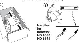
4- Stand Place the stand with the flat side against the support, ensuring that one of the nylon washers is on each side of the stand (follow the drawing).
