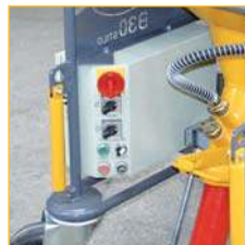
The electrical control panel allows the control of all functions of the machine in a simple way.
